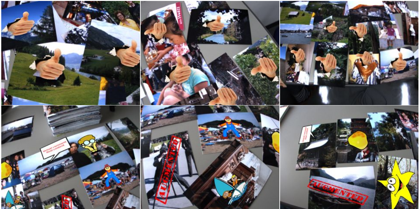
Figure 10: Augmenting multiple objects simultaneously. Our system retrieves, track, and augment the pictures lying on the desk. On the first row, all the objects are augmented with the same virtual content. On the second row, the virtual elements vary from object to object. In these examples, 3 to 6 pictures are tracked and augmented simultaneously.
