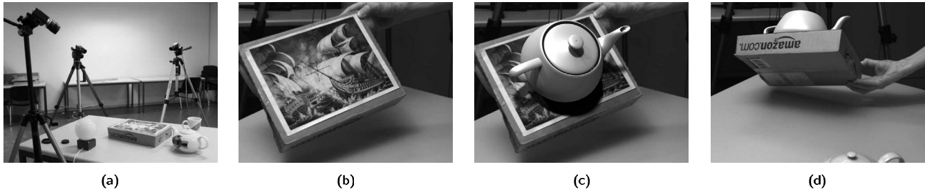
Figure 1: From calibration to augmentation. (a) Our setup. Note the complexity of the ambient lighting. (b) A raw image acquired by one of the cameras. The planar pattern on the box is automatically detected and used for calibration purposes. (c) A virtual teapot has been added. It is properly lit and casts a shadow on the real box. (d) The virtual teapot is still correctly registered and occluded by the box even though the calibration pattern is not visible in this view.
